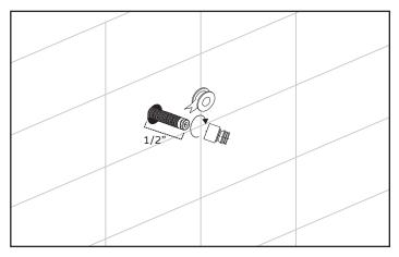
Add plumber's tape to nipple and screw inlet fitting (2) onto nipple (3).
