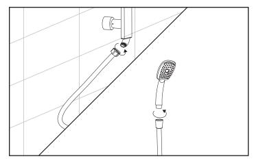
Attach hex head end of hose (13) to swivel joint (11) and tapered end to hand shower (14).
