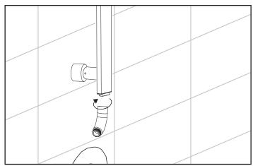
Screw swivel joint (11) onto shower bar.
