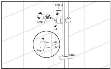
Step1: Slide top pipe onto inlet fitting (2). Step2: Secure with set screws (5). Step3: Slide escutcheon (4) to cover set screws (5).
