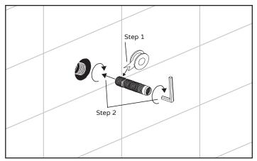
Add plumber's tape to nipple and screw nipple (3) into pipe. Make sure you leave 1/2" off the wall. Use nipple extensions as needed.
