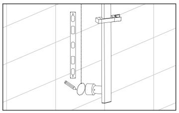
Use level to assure shower pipe is straight. Mark desired location for bottom mount (10).
