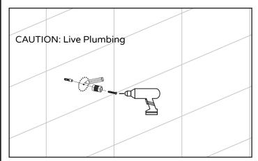
Center mount into the outline of the bottom mount. Mount bottom mount (10) with mounting screw (16).
