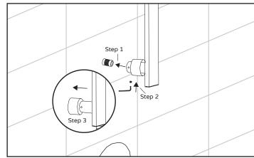
Step1: Slide bottom support over bottom mount (10). Step2: Secure with set screw (5). Step3: Slide escutcheon (4) to cover set screws. (5).
